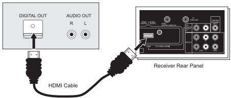
Connect the HDMI Cable from the DIGITAL OUT on the back of your DTV or HDMI device, to the DIGITAL-IN on the back of your television.
